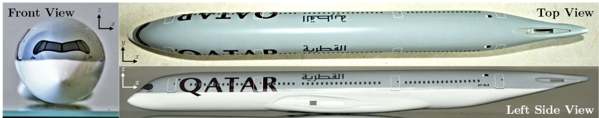
Figure 3. The 2D orthographic projections of the A350-900 fuselage. The x , y and z axes are aligned along the length, width, and height of the fuselage respectively.
